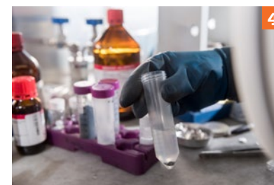
4-5 The resulting alloy sample is then placed in a test tube containing a solvent such as ethanol, where the reactive lithium dissolves out into solution.
