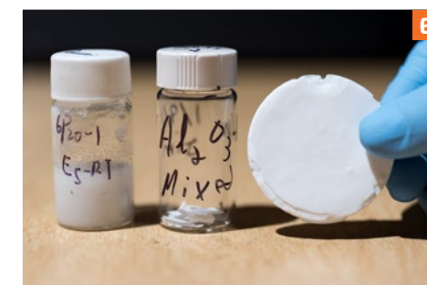
6 The aluminum nuclei left behind seed the growth of aluminum alkoxide nanowires, which can be heated in the open air to form paper-like sheets.
