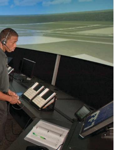
Our \$3.4 million Air Traffic Control Training and Research Facility includes a seamless, 360-degree fiberglass virtual control tower, the only one like it in the world. The facility, 29 feet in diameter, features 10 high-definition digital projectors that create the most realistic tower simulation available today.
