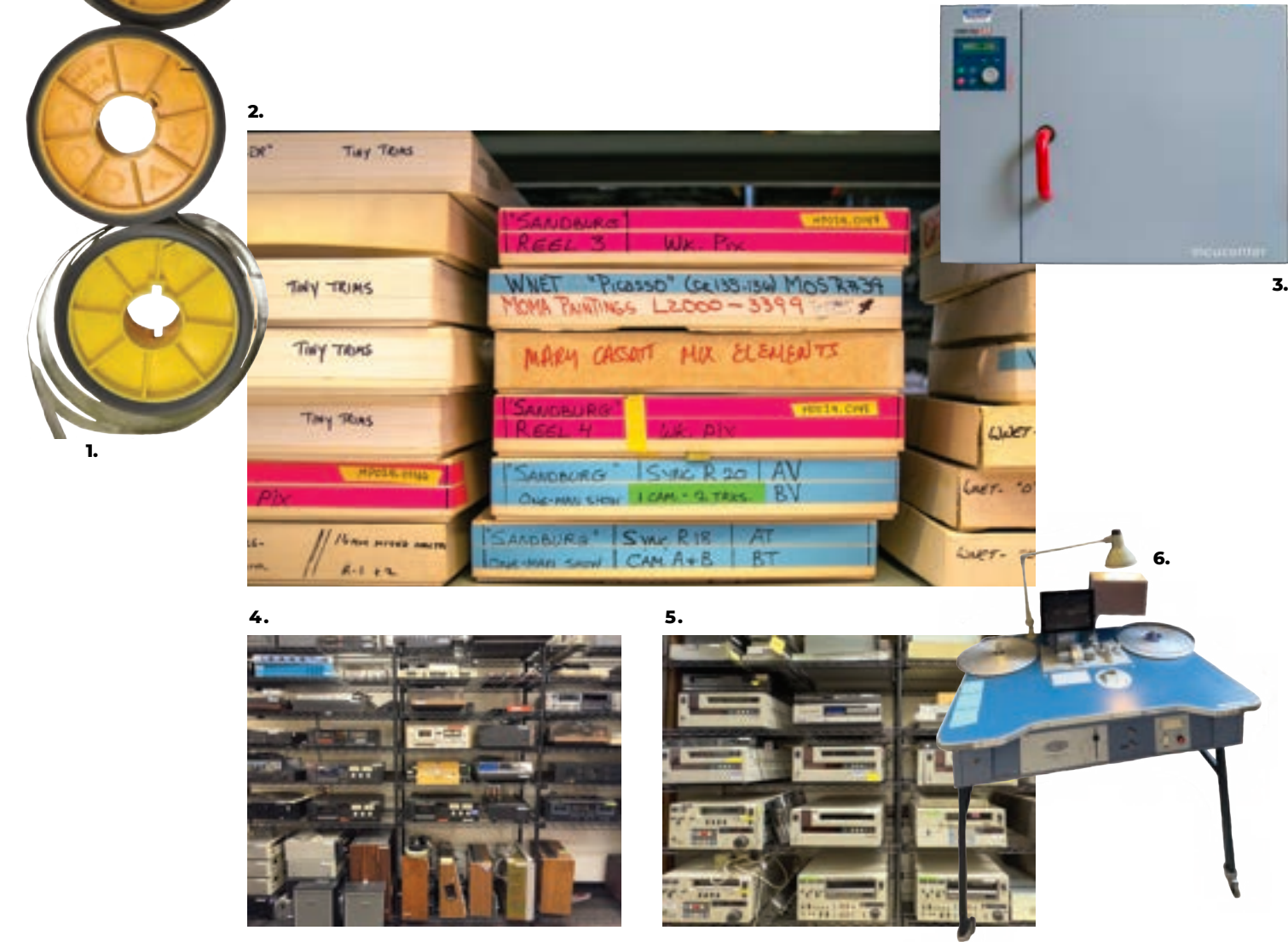
1. These sections of film will be preserved, stabilized, and wound on new cores. 2. The Media Preservation Lab values the importance of preserving metadata, including the information written on these boxes. 3. This incubator is used to dry out damaged film, video, and audio tape that has become sticky over time. 4. A collection of analog audio equipment, including record players, cassette, and reel-to-reel audio players. 5. Several Sony Betacam and U-matic players/recorders line the shelves in the Media Lab. 6. Analog film editing was done on Steenbeck editing tables. The Media Lab uses it to review the content and condition of historic films.
