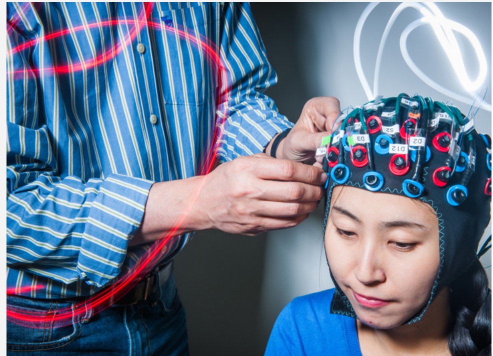
David Boas and his team, including research fellow Xinge Li, can look 5 to 10 mm beneath the skull using functional near-infrared spectroscopy machines which include flexible caps fitted with optodes that transmit and detect light.
