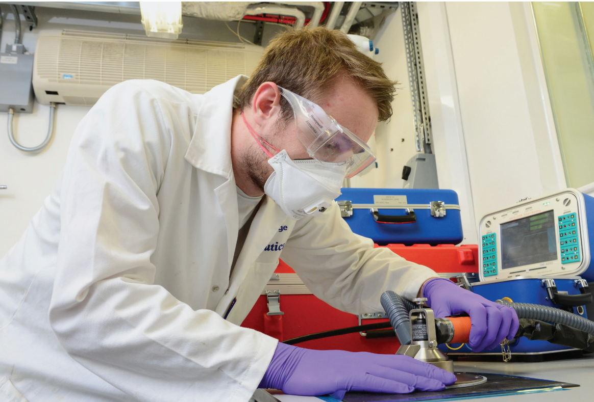
▲ We are developing methods for in-service repair of composite components.
