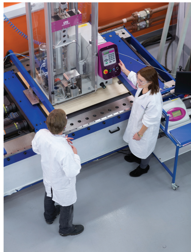
▼ We are investigating the effect of compressive preload on impact resistance of composite structures using our unique impact under load capability.
