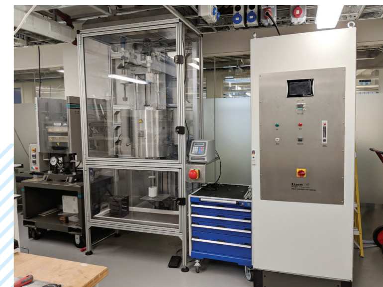
▼ Our furnace for making CNT reinforced light alloys.
