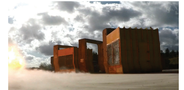
▲ Blast experiment on composite component.
