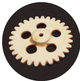
▲ Additive manufactured ceramic composite component.
