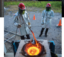
UB geologists make lava for experiments at the Center for GeoHazards Studies in Ashford, NY. The facility provides a rare venue for research on why the interplay between molten rock and water sometimes generates huge explosions and at other times, no damage at all.
